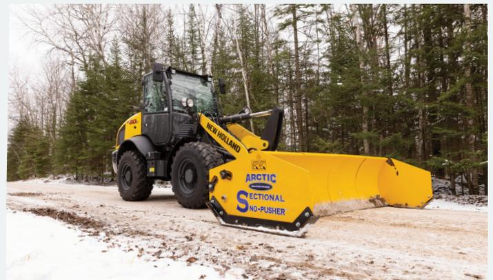
W70C and W80C axles can produce a top speed of up to 25 mph (40kph), able to drive from jobsite to jobsite in many cases eliminating the need for additional transportation with truck and trailer.
