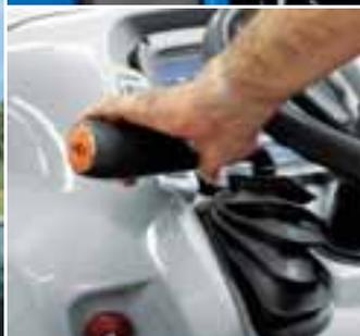
The standard 12x12 synchromesh transmission, with synchronised forward/reverse shuttle further increases the versatility of the TDF tractors, while the optional 20x12 creeper, providing minimum speeds down to 300 m/h at rated engine speed, is ideal for specific applications.
