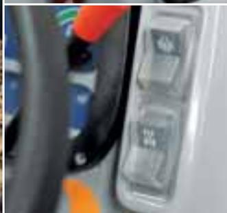
Standard electro-hydraulic control of the four-wheel drive and differential-lock engagement through conveniently located switches.
