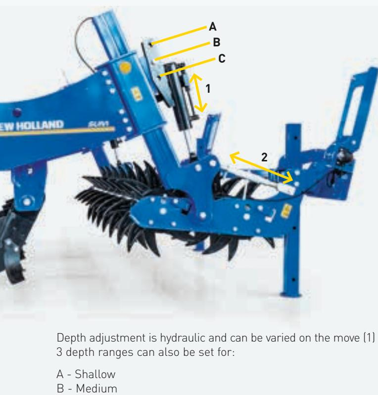
Depth adjustment is hydraulic and can be varied on the move [1]
