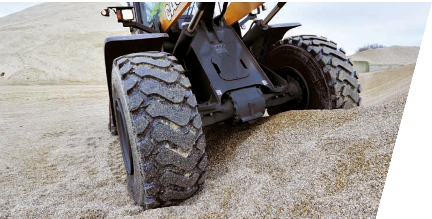
With L5 tyres, needed for work in very abrasive environments, we recommend heavy-duty axles. Solid tires can be retrofitted
