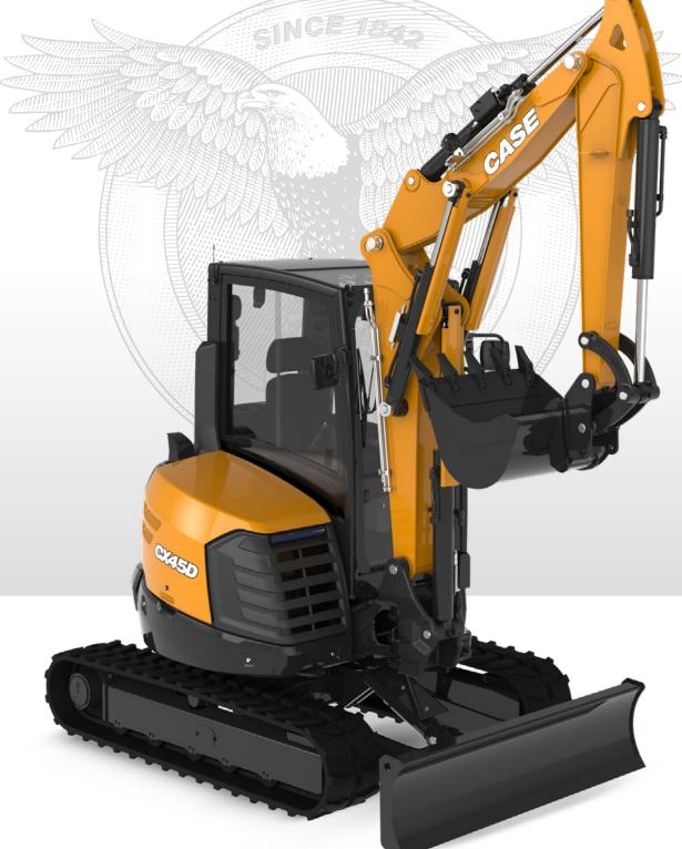
Engine D1803-CR-T Engine power 32.3 kW - 43.3 hp Operating weight 4750 kg
