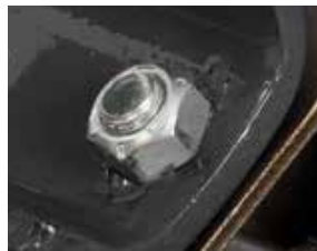
THEIRS: Uneven painted slats which impact torque.
